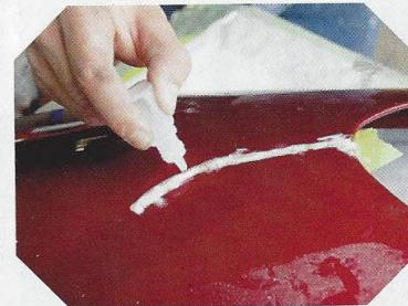
**28** Make sure the powder is completely saturated with hardener.
