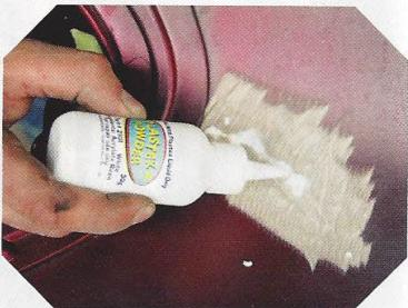
**22** Alternatively, you can sprinkle the powder directly into the crack or hole to be repaired (as long as it can be laid horizontally, so the powder doesn't fall out).
