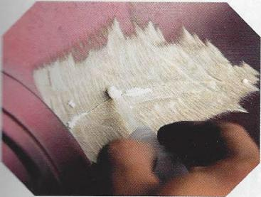
**21** Place the droplet into the crack and let dry.
