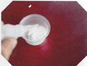
**20** Add a couple drops of hardener to the powder, but don't saturate it completely, as you'll use the applicator tip to pick up a small droplet.
