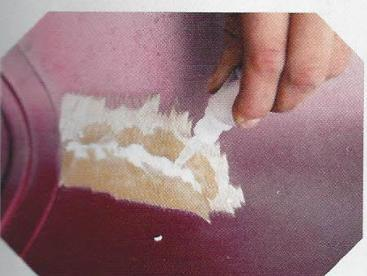
**23** Saturate the powder thoroughly. You don't need to measure the ratio; just make sure it's wetted completely.
