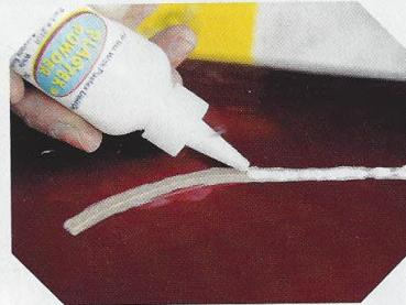
**27** Apply powder (or wet droplets) to the groove in the outer surface.
