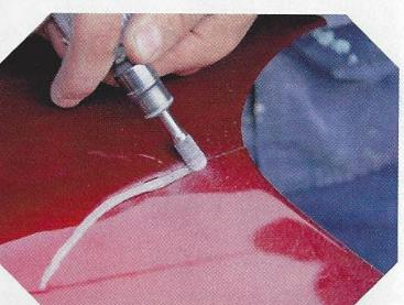
**26** Use a Dremel or other fine grinder to create a groove in the surface. The following steps also apply to repairing crazing or surface cracks on fiberglass.
