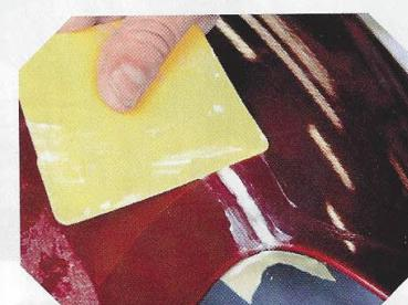
**29** Use a spreader to force the mixture into the groove and even out the surface.
