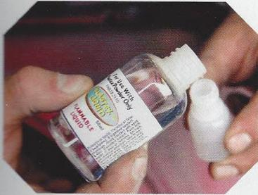
**19** Pour the hardener into a smaller bottle, and cap it with an applicator tip.
