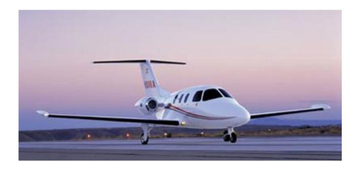
Powered by two Pratt & Whitney Canadian (P&WC) PW6105F turbine engines, the new ECLIPSE 500 VLP (very light jet) delivers 375-ktas performance up to a range of 1,280 nautical miles for less than the price of most used turbo props.
