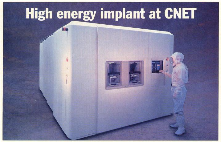
ater this year, Varian will launch formally its latest ion implantation system, E-500. Designed around the needs of some of the world's most advanced process requirements, E-500 is seeking to provide precise solutions to the needs for medium to high energy implantation based on an extension of the already well-established E-220 medium current machine. The Silicon Technology Group at CNET (Centre National d-Études des Télécommunications) in Grenoble is the first European user of this system.
