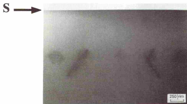
Fig. 19. Cross-sectional transmission electron micrograph of a sample implanted with 10 keV ^{11}\text{B} ions to a dose of 1 \times 10^{13} \text{ cm}^{-2} along [100] and subsequently with 5 \times 10^{14} \text{ cm}^{-2} , 1 MeV silicon ions. The sample was annealed for 10 s at 900 °C followed by annealing for 15 min at 1000 °C. Extended defects ( \phi \approx 0.3 \mu\text{m} ) are observed at a depth of 1 \mu\text{m} below the surface.
