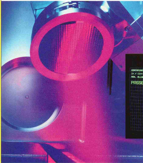
New E500 Ion Implanter automatically ensures beam purity before implantation.
