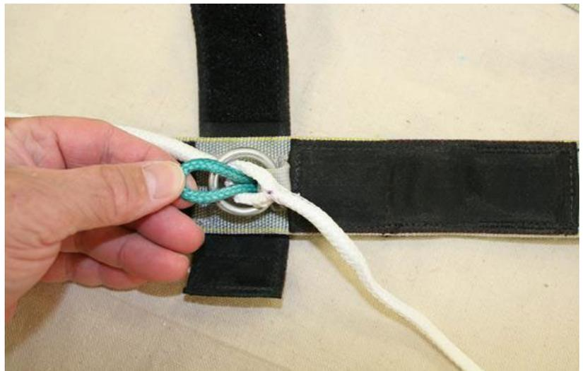
Figure 27. Inspect Brake Locking Loop on each Riser
