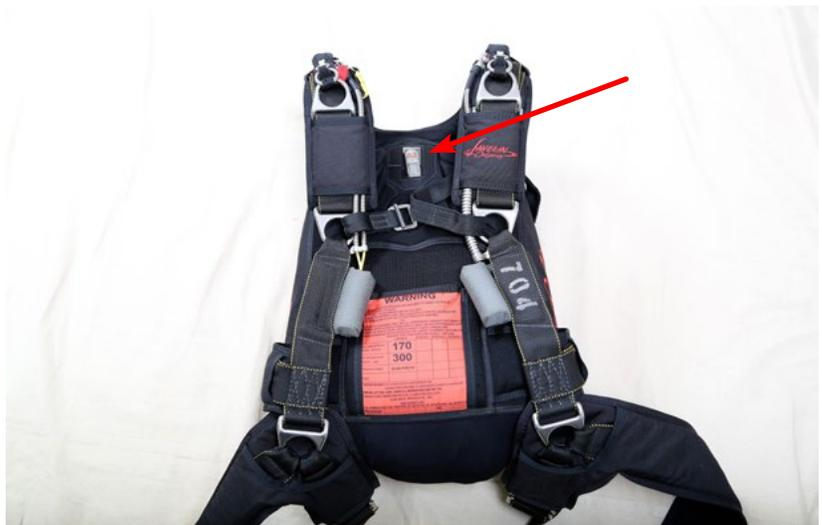
Figure 59. AAD – Properly Calibrated
