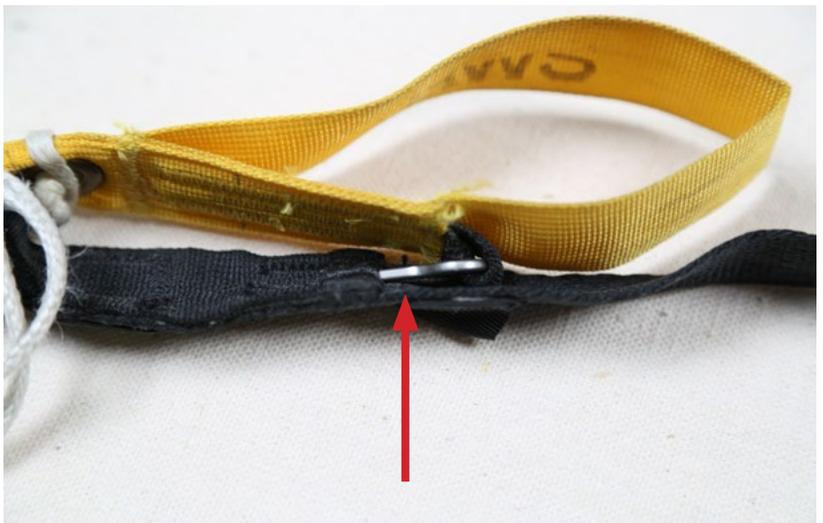
Figure 30. Check Toggle Retention is Secure
