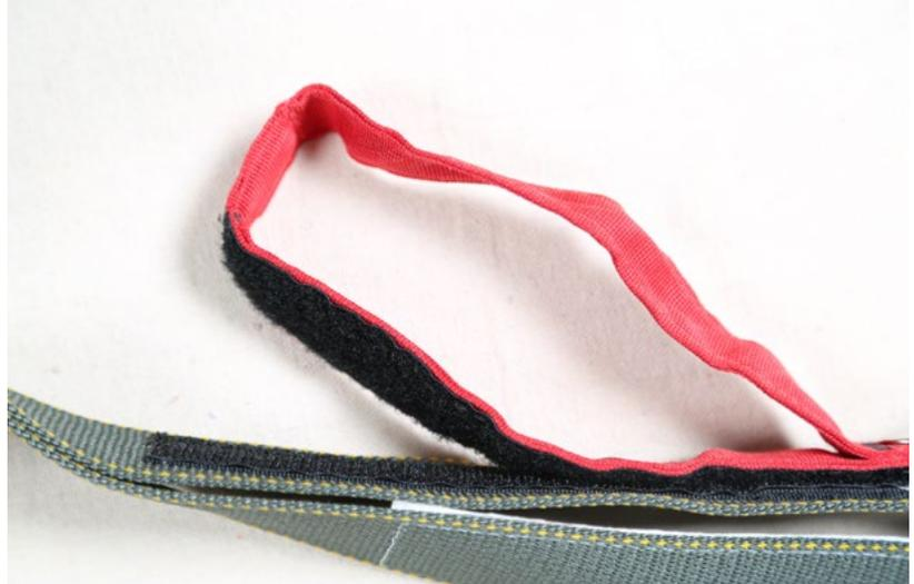
Figure 31. Inspect Velcro Condition
