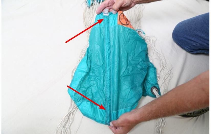
Figure 40. Inspect Channels on Collapsible Slider
