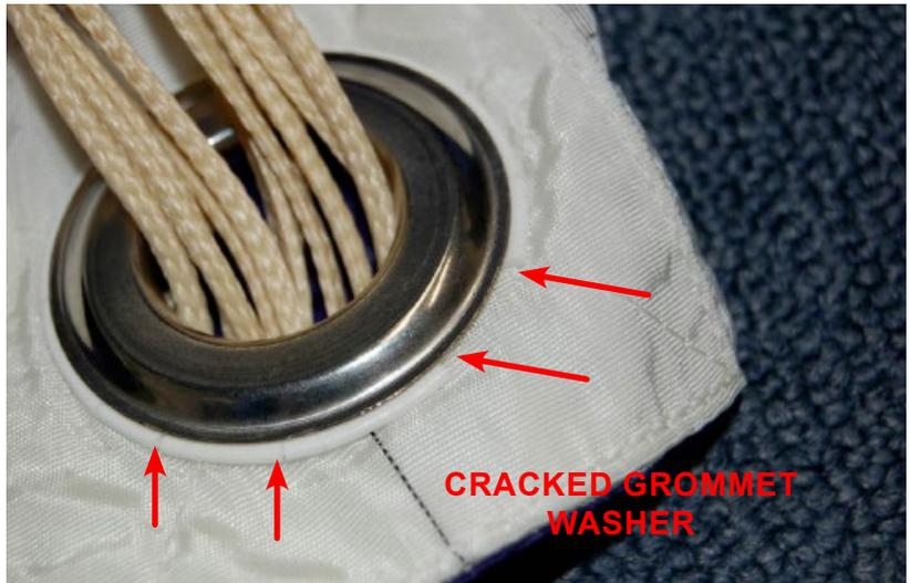
Figure 38. Inspect the Grommet Washer
