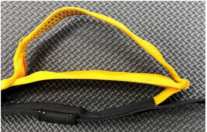
Figure 29. Inspect Tuck Tab Keeper
