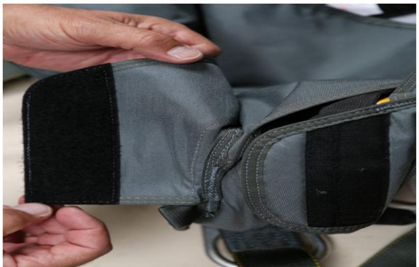
**Figure 10. Check the Condition of the Velcro**
