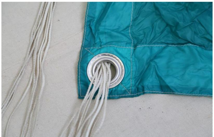
Figure 36. Inspect All Slider Grommets for Damage
