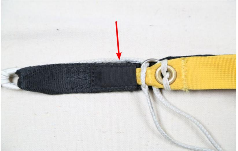
Figure 28. Inspect Toggle Tip Keeper
