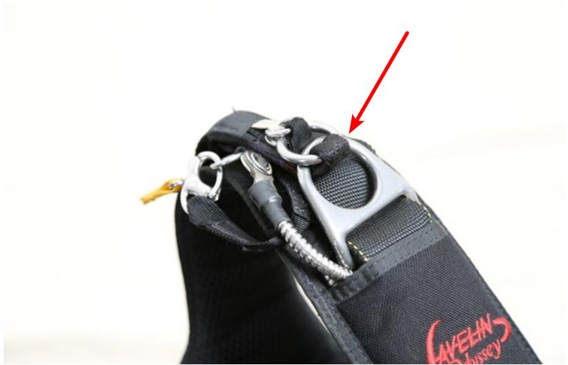
Figure 55. 3-Ring Assembly Check
