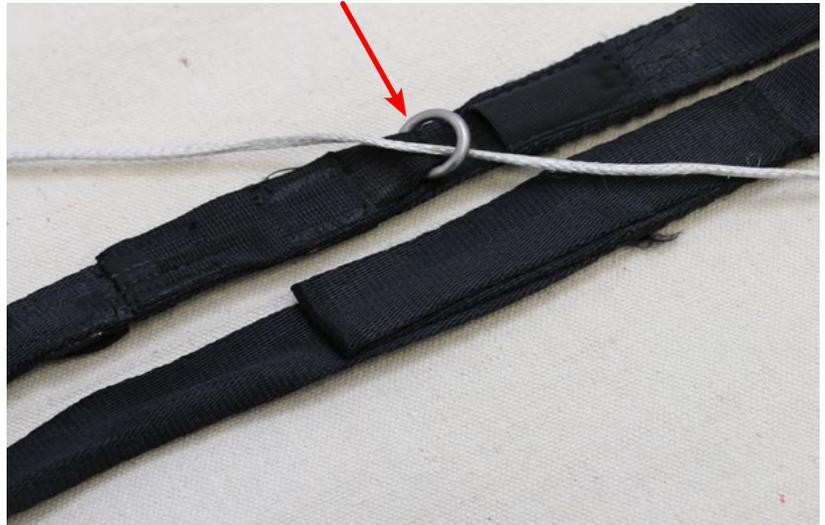
Figure 25. Inspect Guide Rings
