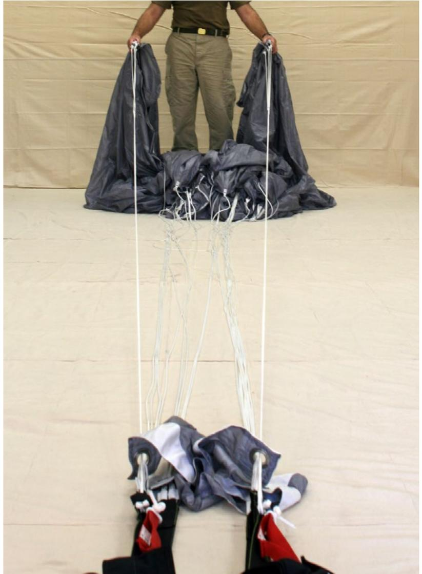
Figure 24. Control Line Check
