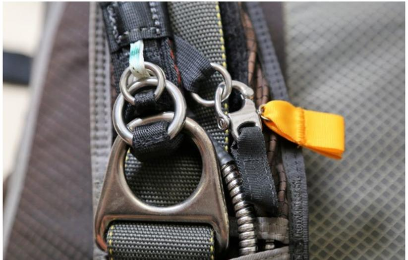
Figure 14. 3-Ring - Properly Assembled
