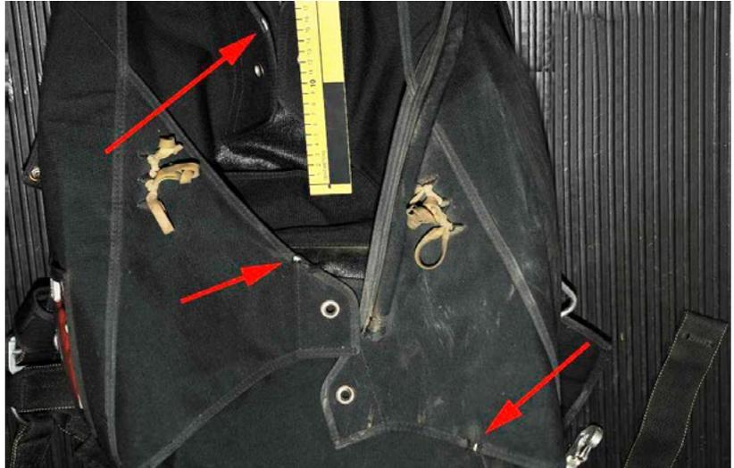
Figure 5. Fabric Abrasion & Exposed Plastic Stiffeners
