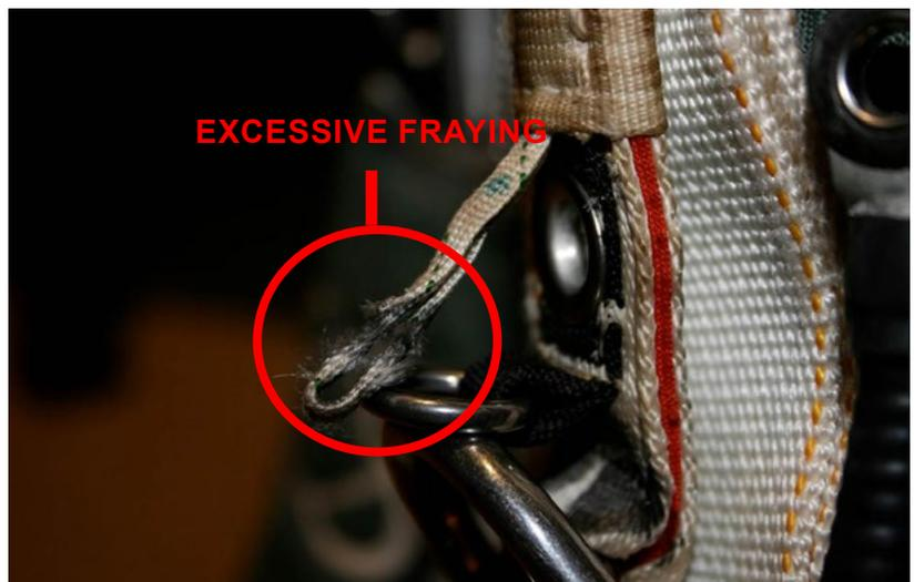
Figure 15. Damaged Locking Loop
