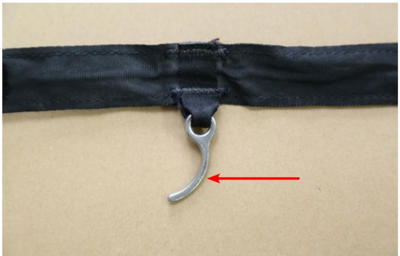
Figure 47. Inspect the Container Closing Pin
