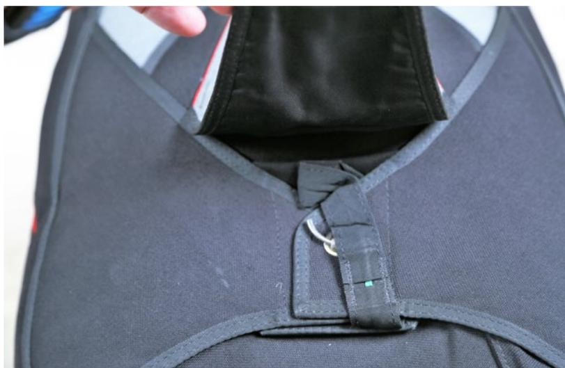
Figure 50. Main Pin and Bridle Check
