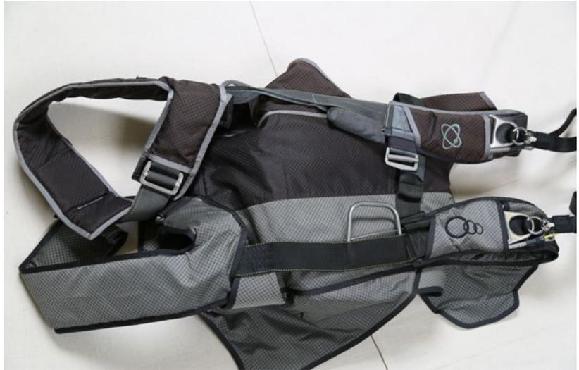
Figure 11. Inspect Harness Webbing for Damage
