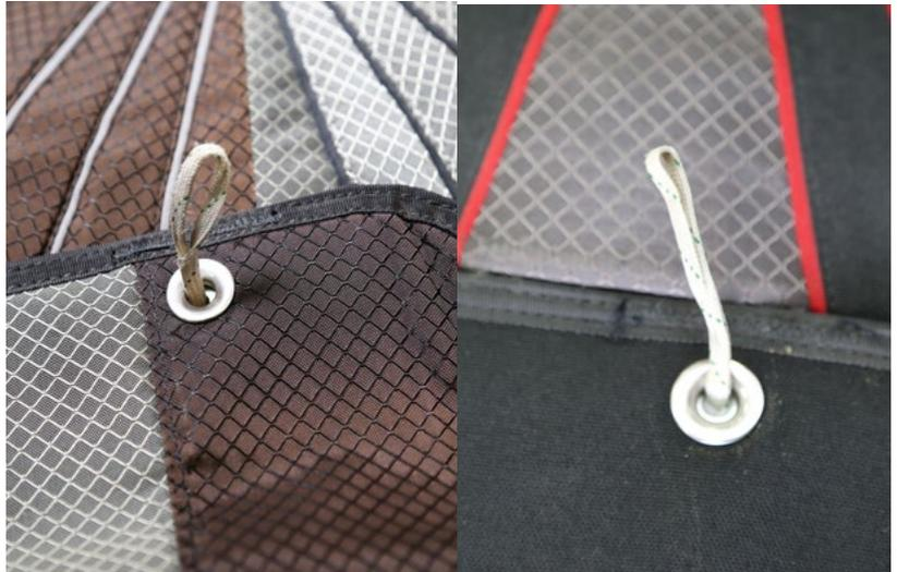
**Figure 8. Inspect The Main Closing Loop**
