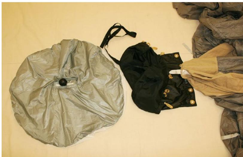
Figure 22. Inspect the Main Pilot Chute
