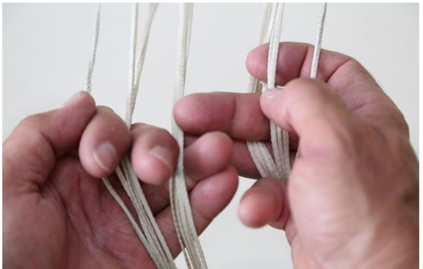
Figure 42. Inspect Condition of Lines
