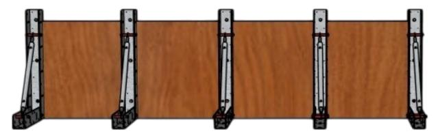
Shown used @ 4' on centre as a prop on existing lumber forms, brackets have screw fixing holes to fix to the forms
