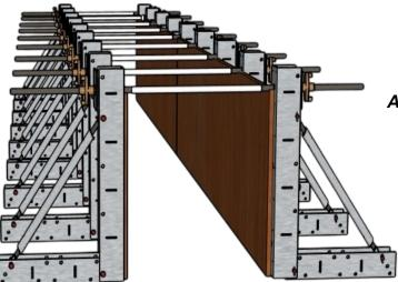
Add tie bars over the top of pours if needed (mot needed up to 4'), they can also be fitted in the pours for wall pours and remove the need for snap ties and give a much better finish
