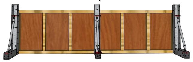
Shown used at 5' on centre as a filler panel & prop on Symons Steelply 2' x 5' panel, brackets have pin & wedge slots that match the steelply, you can use a tie bar over the top of a pour on double sided, Bracket also eliminates the need for snap ties completely
