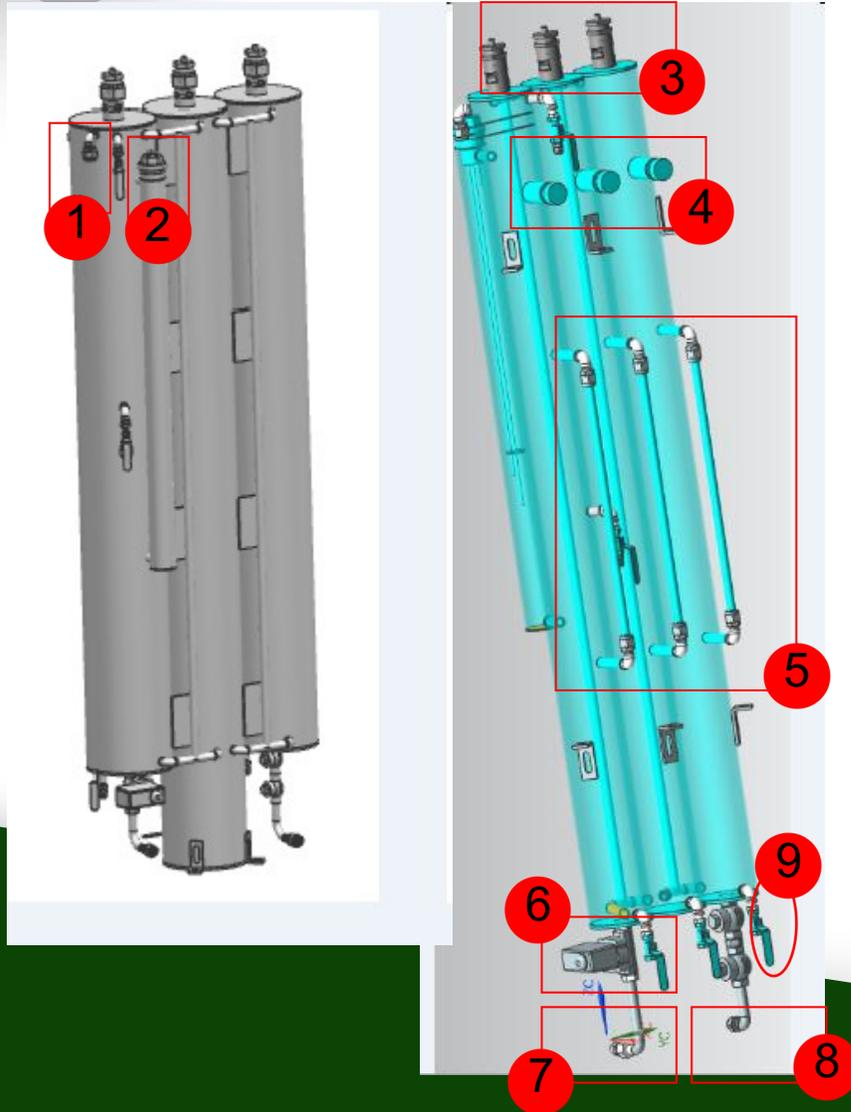
1- Gas gate of anti-backfire tank 2- Water level needle of anti-backfire tank 3-Safety valve 4-Manual filler 5-Transparent liquid level tube
