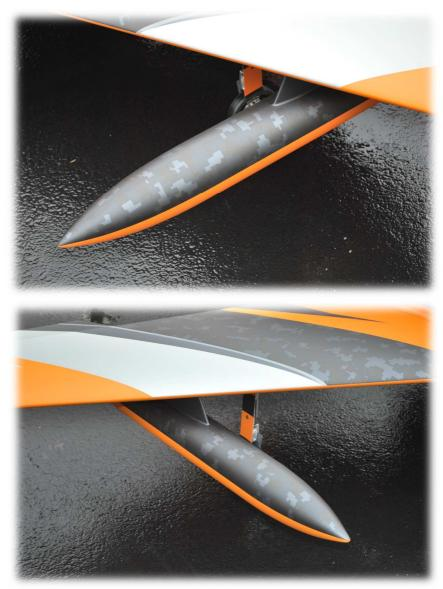
The completed photos demonstrate the importance of getting the surface smooth and eliminating all the paint ridges we had from the masking process.
