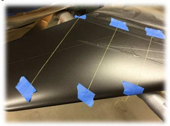
Then as the masks are placed on to the surface it's immediately apparent if they aren't perpendicular to each other.
