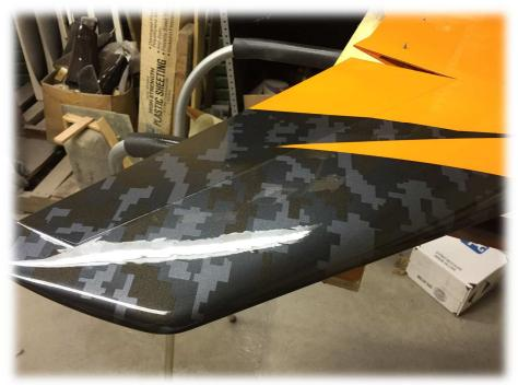
After the clear had a chance to cure I wet sanded (400 grit) it smooth by hand with a sanding block. This sanding leveled out the surface nicely and also removed the 'orange peel' from the clear coat. In this photo the top tank isn't sanded, while the bottom one has been. If you look at the light reflection you can see the smoother surface.
