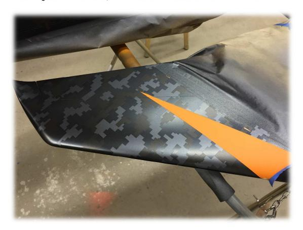
During this step of removing the masks, it's very important to make sure to find and remove them all. If you don't they will be trapped by the clear coat and cause issues when you sand out the clear.
