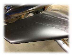
Now the fun starts. How to effectively mask off this area for the digital camo pattern? Well, this is where the computer and computer assisted vinyl cutter becomes your best friend. The random pixel patterns are drawn on the computer and cut by the vinyl cutter out of masking film. The orientation and spacing of the patterns on the sheet isn't critical, in fact if you bunch them up it's a more economical use of the film.
