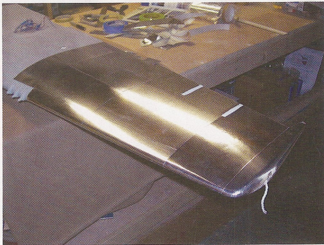
Continue adding panels until the wing is covered
