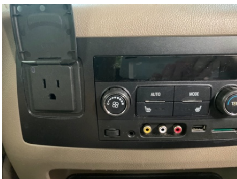
Figure 4: 120Vac outlet (source David Tuttle)
