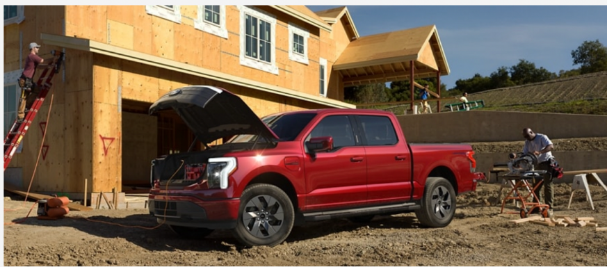
Figure 6: Powering Loads with V2L (source Ford)
