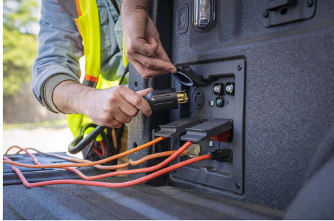
Figure 5: 120Vac and 240Vac receptacles (source Ford)
