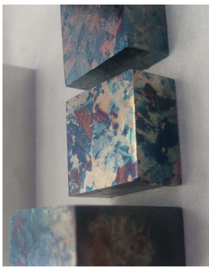
Extreme surface oxidation
