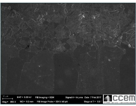
Many areas of the interface were not suitable for a liftout due to the roughness of the interface
