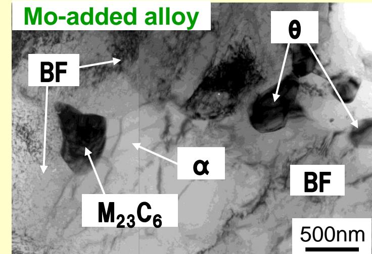
BF: Bainitic Ferrite MA: Martensite-Austenite constituent α: Ferrite θ: Cementite  $M_{23}C_6$  carbide
