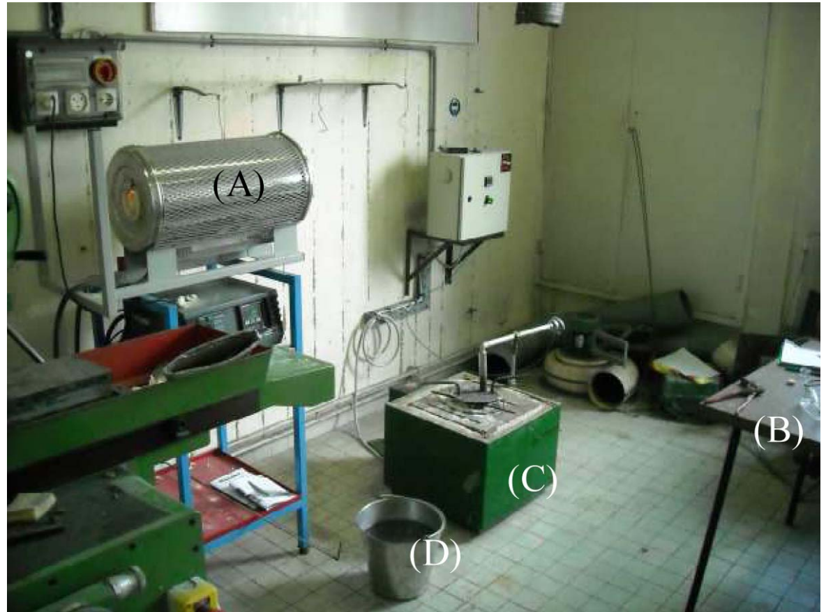
(A) carbolite tubular furnace (B) clamp used to break glass capsule before salt bath treatment (C) barium chloride salt bath (D) water quenching bucket.
