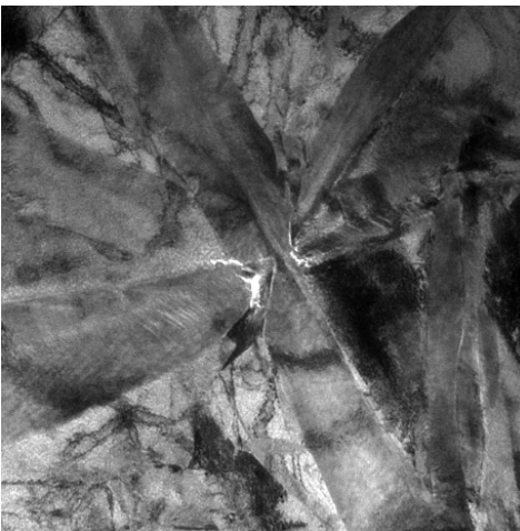
Fe 1.67% C (HT 10 min @ 1100°C, A. Stormvinter - KTH)
