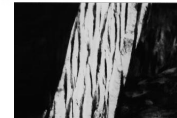
Fig. 5.80 Massive \alpha in an Fe-0.002 wt% C quenched into iced brine from 1000 °C. Note the irregular \alpha/\alpha boundaries. (After T.B. Massalski in Metals Handbook , 8th edn., Vol. 8, American Society for Metals, 1973, p. 186.)
