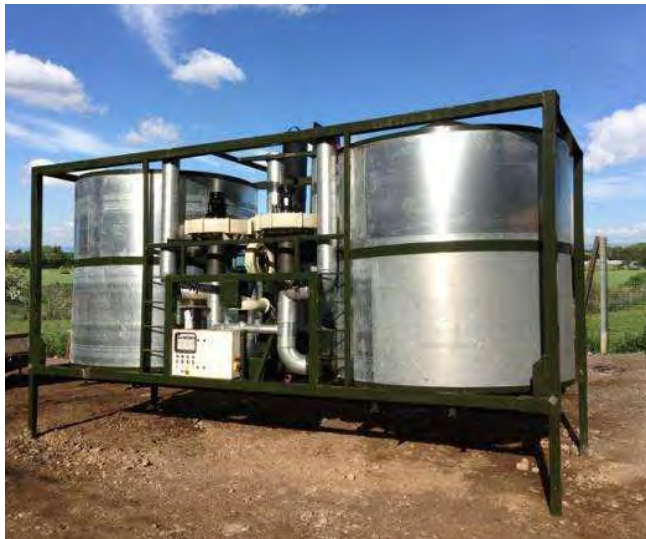
Semi-continuous kiln for IBERS, Institute of Biological, Environmental and Rural Sciences, Aberystwyth University (2016)
