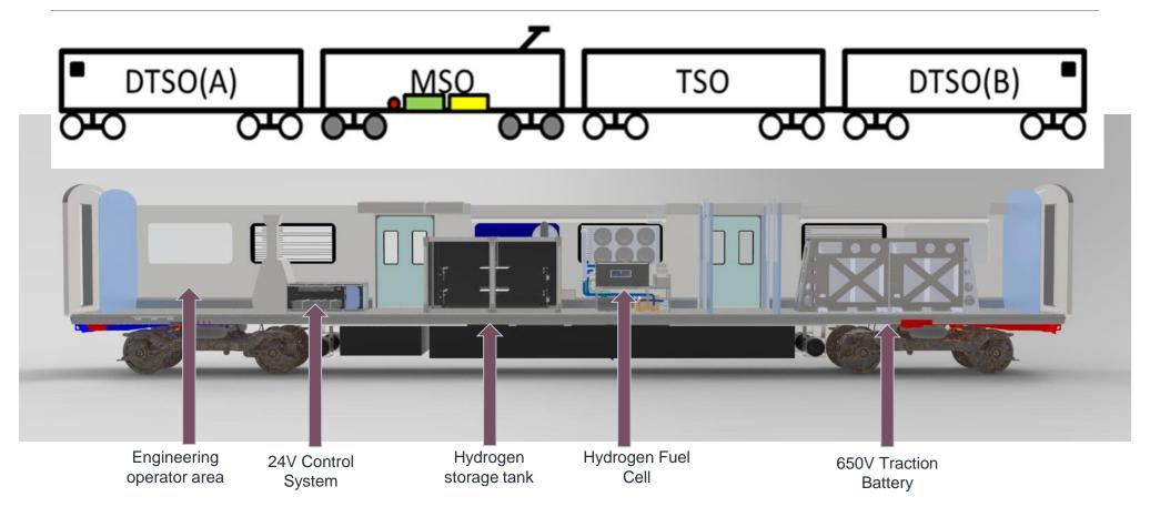
The MSO vehicle needed its seats and interior fittings removed to house the HydroFLEX system components
