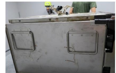
Condition of left and right faces of module after the nail penetration test
