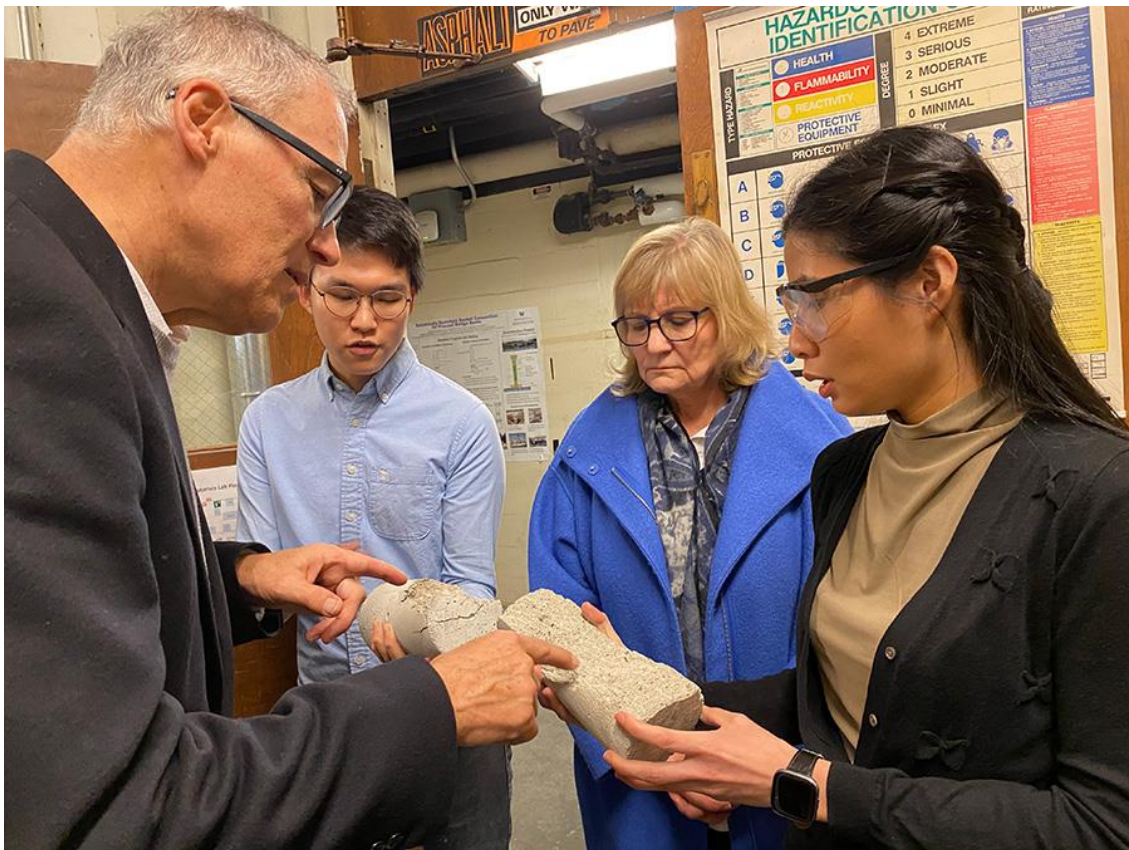
MSE master's students Kunthea Deng and Renjie Song show Gov. Jay Inslee and his wife, Trudi, how samples of zeolite concrete fractured in compression tests.
