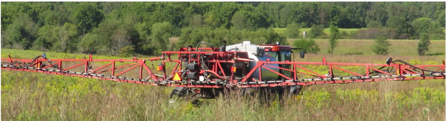
Boom sprayer applying herbicide to a field. Photo Credit: Robert Suseland
