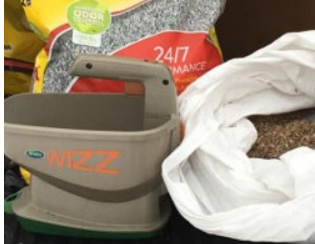
Battery operated handheld broadcast spreaders work well for seeding small areas. Photo Credit: Robert Suseland
