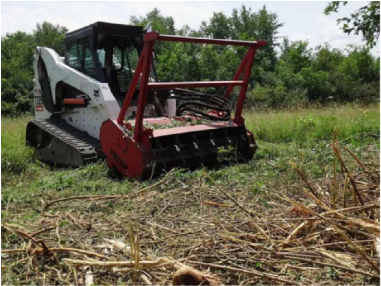
A forestry mower levels all vegetation, making follow up treatments easier. (Photo credit: Penn State Extension)
