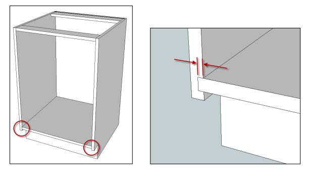
For bottom panels that fit into rabbets in the side panels, enter the depth of the rabbet that will be cut into the side panels.
