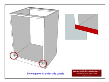
• Cell L34 (Cell L24 Frameless) Select MITER TO SIDE PANELS if you want the outboard edges of the bottom panel and the lower edges of the side panels mitered 45 degrees.
