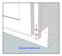
Cell S73 (Face Frame version only) For OVERLAY requirements: enter the amount of overlay that is required on the center rails (NOTE: center rails are applicable only on some cabinet configurations).
