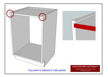
• Cell L32 (Cell L22 Frameless) Select RABBET SIDE PANELS if you want the top panel to fit into a rabbet that is cut along the top edge of the side panels. Use the "Set-Up Values" to specify the rabbet depth.
