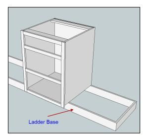
• Cell S44 (Face Frame version only) If a LADDER BASE is selected, this dimension is measured from the floor to the lower edge of the side panels or the bottom panel (whichever is lower).
