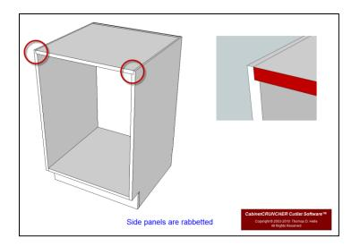
• Cell L32 (Cell L22 Frameless) Select RABBET TOP PANEL if you want the side panels to fit into a rabbet that is cut along the outboard edges of the top panel. Use the "Set-Up Values" to specify the rabbet depth.
