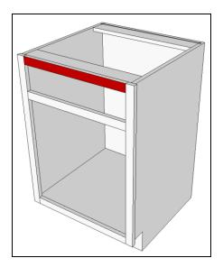
For "BUILT-IN", "FREE-STANDING" and "WALL CABINETS", enter how far the lower edge of the top rail will extend below the lower surface of the top panel. Enter 0 if you want the lower edge of the top rail to be flush with the lower surface of the top panel.
