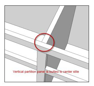
• Cell L39 (Face Frame version only) Select DADO CENTER STILE if a dado will be cut into the back surface of the center stiles to accommodate the vertical partition panels.
