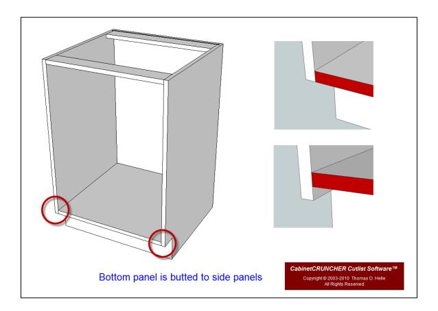
• Cell L34 (Cell L24 Frameless) Select DADO SIDE PANELS if you want the bottom panel to fit into dado's that are cut into the side panels. Use the "Set-Up Values" to specify the dado depth.
