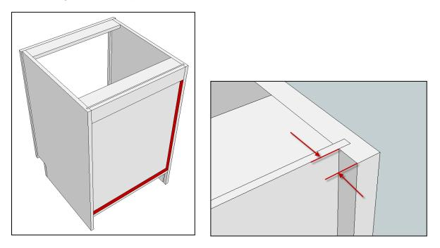
If Cell L35 (Cell L26 Frameless) is set to "RABBET SIDE PANELS", enter the width of the rabbet along the back edge of the side panels (see below).
