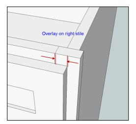
**Cell S70 (Face Frame version only)** For OVERLAY requirements: enter the amount of • overlay that is required on the center stiles (NOTE: the center stiles are applicable only on some cabinet configurations).
