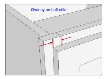
• Cell S69 (Face Frame version only) For OVERLAY requirements: enter the amount of overlay that is required on the right stile.
