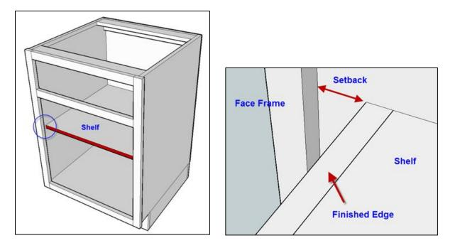
• Cell N53 (Face Frame version only) If the shelves require an applied hardwood trim or edge band on the front edge of the panel, enter the thickness of the trim material.
