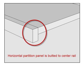
• **Cell L41 (Face Frame version only)** Select **DADO CENTER RAIL** if a dado will be cut into the back surface of the center rails to accommodate the horizontal partition panels.
