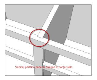
• Cell N39 (Face Frame version only) Enter the depth of dado that will be cut into the face frame center stile to accept the vertical partition panel.
