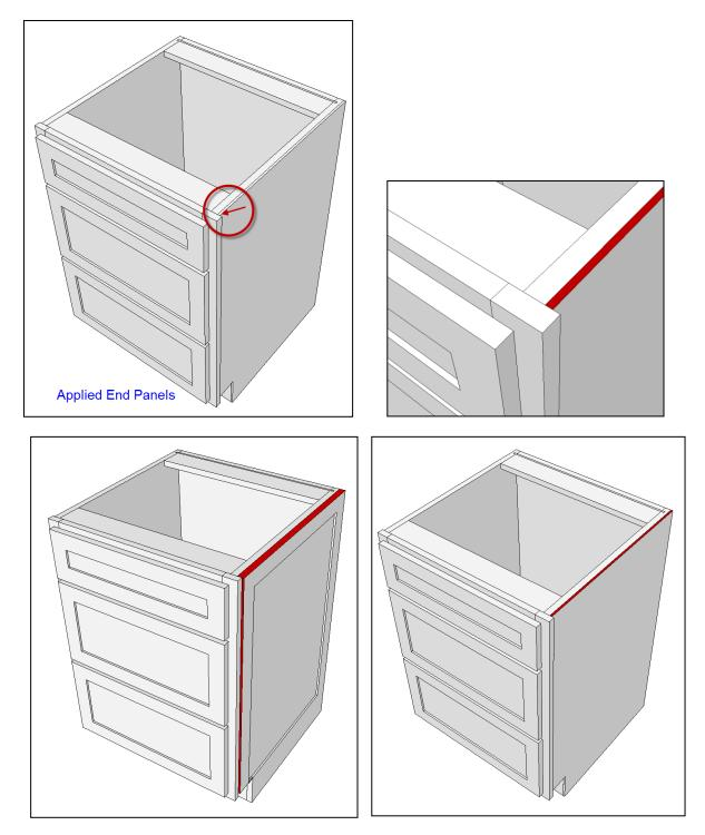
**IMPORTANT:** The total finished width of the cabinet is typically the width of the face frame however, if you are installing applied end panels (refer to quantities in Cell H91 and H92), and if the thickness of the applied end panels extends beyond the face frame stiles, then the finished width of the cabinet will be measured from the outer surfaces of the applied end panels.
