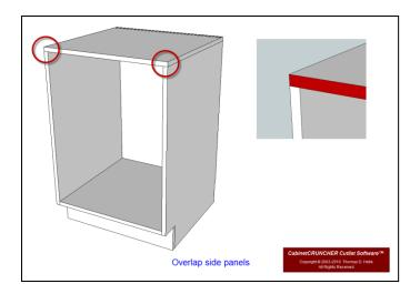
• Cell L32 (Cell L22 Frameless) Select MITER TO SIDE PANELS if you want the outer edges of the top panel and the upper edges of the side panels mitered 45 degrees.
