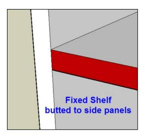
• Cell L50 (Cell L48 Frameless) Select DADO SIDE PANELS if you want the shelf to fit into dados that are cut into the side panels. Use the "Set-Up Values" to specify the dado depth.
