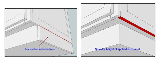
**EXAMPLE:** If you enter 0, the height of the applied end panel will equal the length of the face frame stile. If you enter a dimension that is larger than 0, the height of the applied end panel will increase by the amount entered. If you enter a negative value, the height of the applied end panel will decrease by the amount entered.
