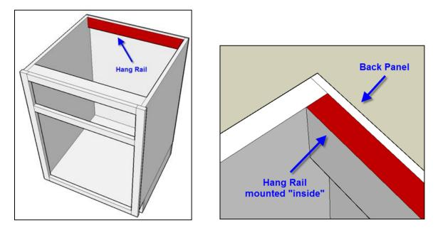
• **Cell L55** Select **INSTALL OUTSIDE** if the hang rail will be installed on the back of the cabinet behind the back panel.
