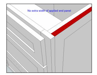
If you enter 0 in this setting, the width of the applied end panel is measured from the back surface of the face frame stile to the back edge of the cabinet. If you enter a dimension that is larger than 0, the width of the applied end panel will increase by the amount entered.
