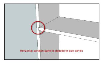
• **Cell N40** If the partition panel will fit into dados that are cut into the side panels, enter the depth of dado.
