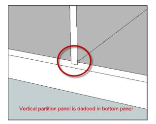
• Cell N38 (Cell N29 Frameless) Enter the depth of dado that will be cut into the top and/or bottom panel to accommodate the vertical partition panel.
