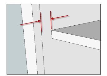
• Cell N41 (Face Frame version only) Enter the depth of dado that will be cut into the face frame center rails to accept the horizontal partition panels.
