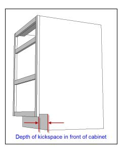
• Cell N47 (Cell N43 Frameless) Enter the desired depth of the kick-space on the left side of the cabinet. This is the distance from the outer surface of the left side panel to the pedestal base.
