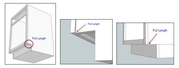
Select **FLUSH BOTTOM PANEL** if you want the bottom edge of the side panels to be flush with the lower surface of the bottom panel.
