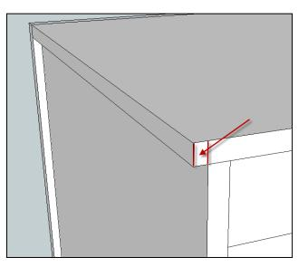
• Cell N33 (Cell N23 Frameless) Specify how far the upper surface of the top panel is located from to the top edge of the side panels.
