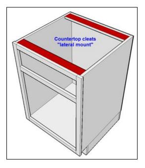
• Cell L56 (Face Frame version only) Select FORE & AFT MOUNT if you want the cleat to extend from the front to the back of the cabinet. NOTE: if a hang rail is installed along the top back edge of the cabinet, the length of the countertop mounting cleat will be shortened by the thickness of the hang rail. In other words, the hang rail will be installed behind the cleat.
