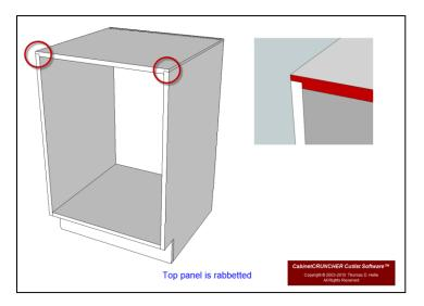
• Cell L32 (Cell L22 Frameless) Select OVERLAP SIDE PANELS if you want the top panel to extend over the top of the side panels. Use the "Set-Up Values" to specify how far the top panel will extend over the outer surface of the side panels.
