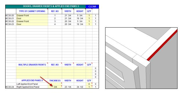
**IMPORTANT:** The total finished width of the cabinet is typically the width of the face frame however, if you are installing applied end panels (refer to quantities in Cell H91 and H92), and if the thickness of the applied end panels extends beyond the face frame stiles, then the finished width of the cabinet will be measured from the outer surfaces of the applied end panels.
