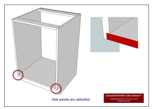
Cell L34 (Cell L24 Frameless) Select RABBET BOTTOM PANEL if you want the side panels to fit into a rabbet that is cut along the outboard edges of the bottom panel. Use the "Set-Up Values" to specify the rabbet width.
