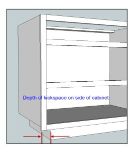
Enter 0 if you want the pedestal base to be flush with the outer surface of the left side panel.
