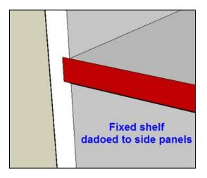
• Cell N50 (Cell N48 Frameless) If the shelves will fit into dados that are cut into the side panels, enter the depth of dado.
