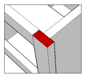
Select **DADO LEFT/RIGHT STILES** if a dado will be cut on the back surface of the left and right stiles to accommodate the left and right-side panels.
