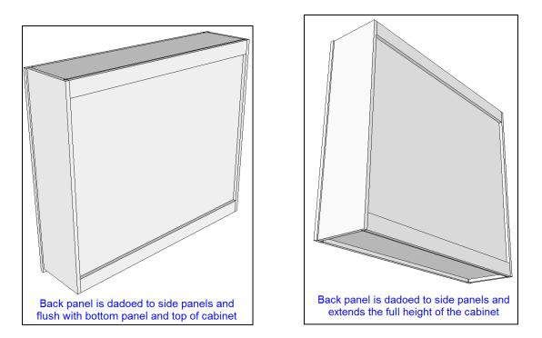
Cell L35 (Cell L26 Frameless) Select RABBET SIDE PANELS if you want the back panel to fit inside rabbets that are cut along the back edge of the side panels. Use the "Set-Up Values" to specify the depth of the rabbet in the side panels.
