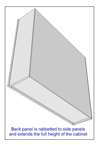
• Cell N35 (Cell N26 Frameless) Enter the depth of dado or rabbet that will be cut along the back edge of the side panels to accommodate the back panel.
