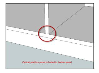
Cell L38 (Cell L29 Frameless) Select DADO TOP/BOTTOM if you want the top and/or bottom edges of the center vertical partition panel to fit into dados that are cut into the top and/or bottom panel
