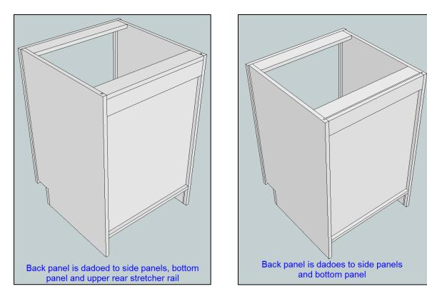
For butted back panels: select **FLUSH BOTTOM PANEL** if you want the back panel to be flush with the top of the cabinet case and flush with the lower surface of the bottom panel. Select **FULL HEIGHT** if you want the back panel to be flush with the top and bottom of the cabinet.
