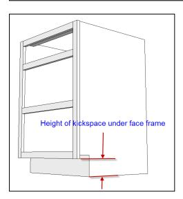
**IMPORTANT:** (Face Frame version only) If this cell is RED, change this setting to 0, or change the base setting in Cell L45, or change the bottom panel setting in Cell L34. Reason: The bottom panel setting that you selected in Cell L34 cannot be installed if you are using a "NO BASE" setting in Cell L45 and the height of the kickspace in Cell N45 is greater than 0.
