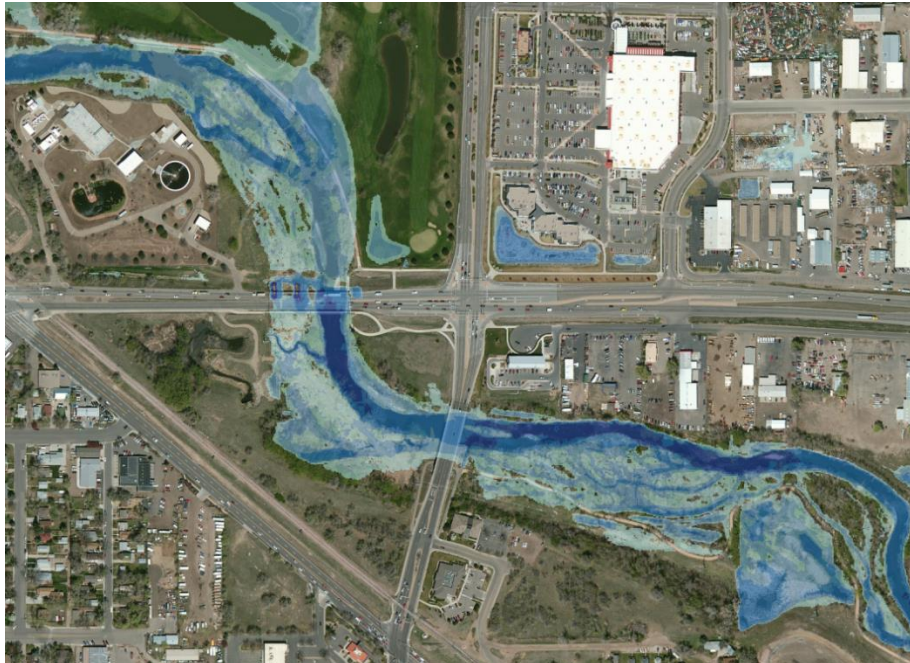
Figure 4.4b: The five-year water surface extent from the Woodward campus to upstream of the Timnath Canal Diversion (lower end of reach 11 and upper half of reach 12) shows a less entrenched channel with a better-connected floodplain.
