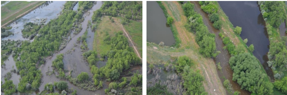
Figure 5.10: In the Plains zone the river has some opportunity for good connectivity with the floodplain which results in higher function through the system and allows for periodic flooding of the riparian zone (left). However, through much of the Plains zone the channel is continues to be highly confined by ponds and berms on either side drastically altering its function (right).
