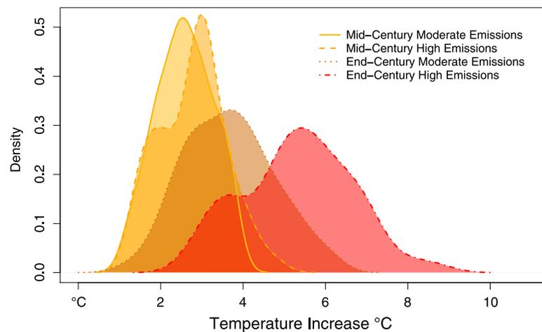
**Figure 3.** Probability density functions of Upper Colorado River Basin temperature projections for midcentury and end-century under moderate (SRES A1B and RCP4.5) and high (SRES A2 and RCP8.5) emissions.
