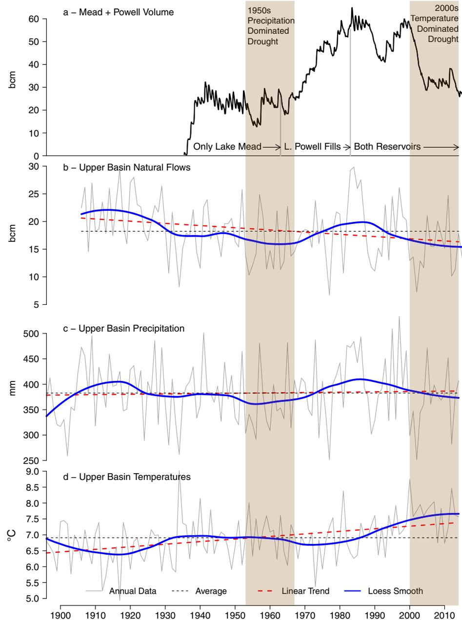
**Figure 2.** (a) Lakes Mead and Powell combined monthly contents. Upper Basin annual Colorado River (b) runoff at Lees Ferry from 1906 to 2014, (c) precipitation and (d) temperatures from 1896 to 2014. Mead first filled in 1935, Powell in 1963 (supporting information Text S1). Two 15-year drought periods, 1953–1967 and 2000–2014, are highlighted and discussed in main text.
