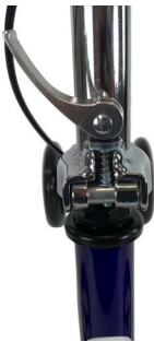
Raise the clamp into the “U” shaped slot
