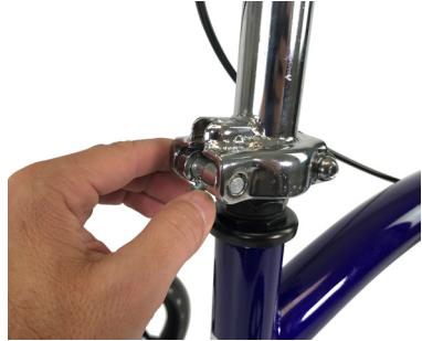
Raise steering column and release the pin
