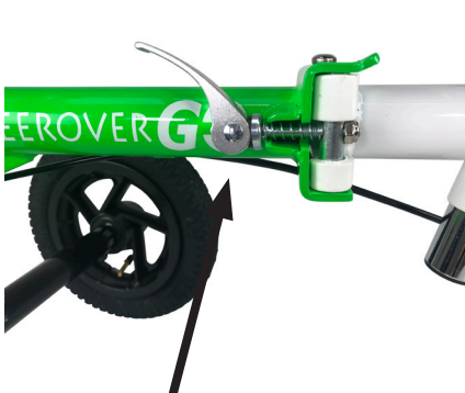
Secure the hinge pin into the “U” slot
