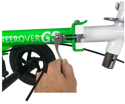
Press lever down firmly until locked
