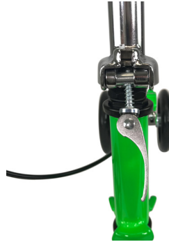
Raise steering column and release the pin
