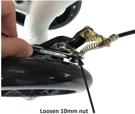
Loosen 10mm nut
