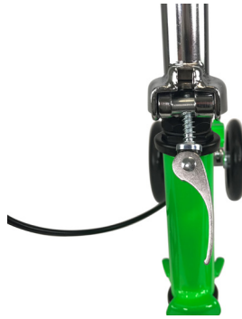
Raise steering column and release the pin
