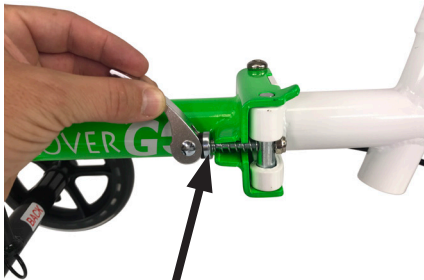
Secure the hinge pin into the “U” slot
