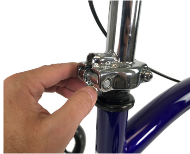
Raise steering column and release the pin
