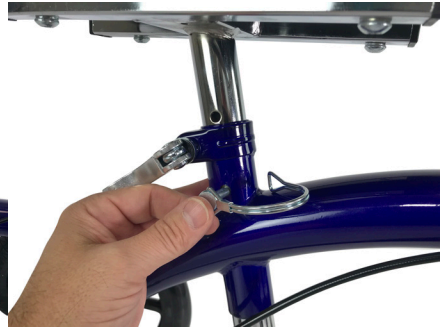
Insert the locking pin through the aligned holes
