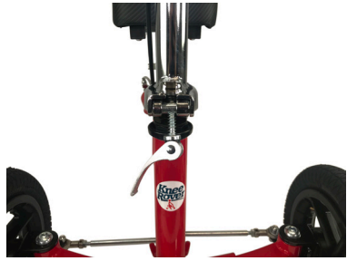
Raise steering column and release the pin
