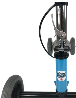
Raise the clamp into the “U” shaped slot
