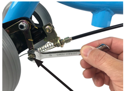
While holding the brake cable, retighten the 10mm nut
