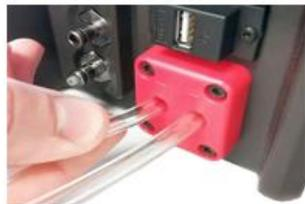
If using DVT, fully insert open end of tubing into DVT connector on front of machine.
