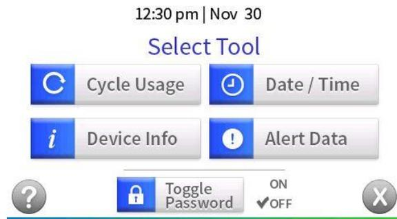
The Cycle Use Information History screen can be reached by selecting the “Cycle Usage” button. It will display the past cycles run on the unit which may be scrolled through using the arrows on the right of the screen. Additionally, there will be a “Back” button to return you to the Select Tool screen and a “Delete?” button. The “Delete?” button will prompt an alert to confirm the previous cycle’s information is deleted.
