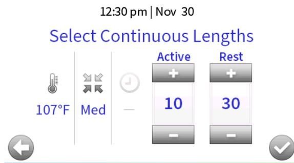
If you have already selected a temperature lower than 40°F or higher than 107°F, or a compression level of ‘High’ while programming a ‘Continuous’ treatment, the software will automatically adjust the temperature and compression to a more conservative choice; 40°F for a cold cycle, 107°F for a warm cycle, and Medium pressure. A continuous cycle cannot be run outside of these parameters.
