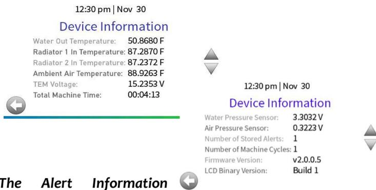
The Device Information screen can be reached by selecting the “Device Info” button. This screen will display a variety of metrics about the unit and its environment. You may navigate through these metrics using the “Up” and “Down” arrow buttons on the right of the screen. There will also be a “Back” button to return to the Select Tool screen.
