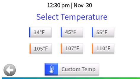
When the “Add 2nd Cycle” button is selected, the unit will present the ‘Select Temperature’ screen. The purpose of this button is to program a second cycle that will initiate at a future date.
