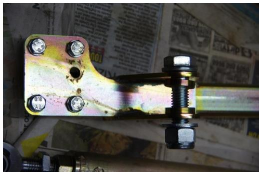
The opposite end of the rod is bolted to this bracket which forms one end of the cross brace and is bolted to the chassis. This arrangement allows the rod to follow the vertical movement of the axle.
