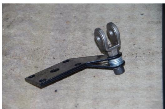
Most other kits have the rod clamped to the spring but there are possibly some disadvantages to this. The SSL kit uses this bracket to attach the rod to the spring. The axle is clamped on to the top of the spring by two large 'U' bolts which are attached to a plate under the spring. By undoing the four 'U' bolt nuts this bracket can be substituted for the plate. The swan neck end of the rod is then bolted to this bracket. This
