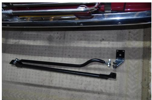
This picture shows the components of the kit laid out at the back of the car as they would be installed. The curved end of the rod will arch over the fuel pipe exiting the fuel tank on the off side. This end of the rod will attach to the bracket which in turn is bolted to the cart spring. The rod is positioned behind the back axle and differential. The other end of the rod attaches to a cross brace bolted to both sides of the chassis behind the axle but in front of the petrol tank.
