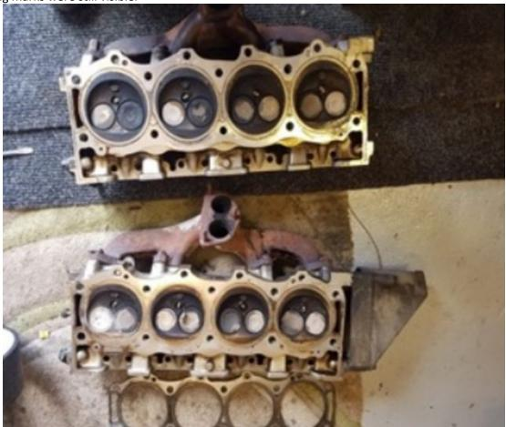
The heads were cleaned and all found to be in very good condition with very little carbon deposits on the valves no oil burns or marks on the valve stems so I decided not to decoke the valves as they were clean and the seats in good condition and I thought why fix what ain't broken.
