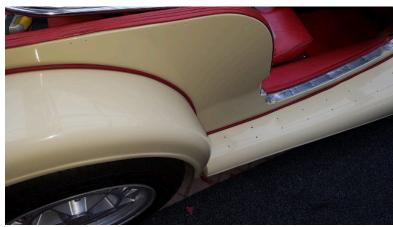
I used rubber gasket between the inner and outer wings with new wing beading that I had made for me to match the upholstery and I think it has made a good contrast with the cream paint work.
