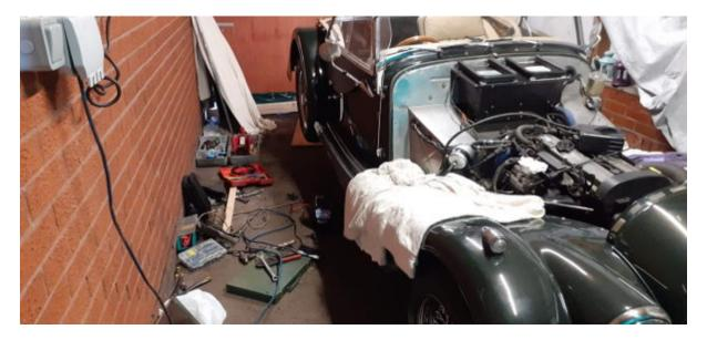
I reassembled all the ancillaries with stainless steel nuts, bolts and screws where possible. The bonnet was finally refitted and the radiator filled with water / anti-freeze. Job Done!
