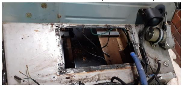
At this point I decided to take everything off the bulkhead so I could give it a good polish at the same time. Then almost standing on my head inside the car with my back cramping up I managed to undo the bolts holding the heater in. Once the heater was free, I lifted it out through the bulkhead.
