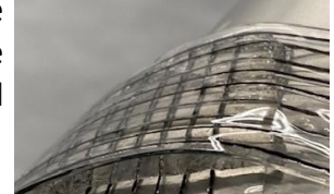
Safety: Tactile TouchSkin™ on robot arm
