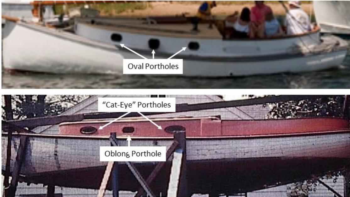
**Figure 9:** Comparisons of cabin and porthole modifications
