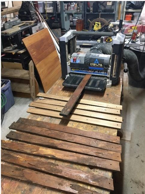
**Figure 15:** Teak salvaged from the rotted deck section and elsewhere was recycled for the hatch
