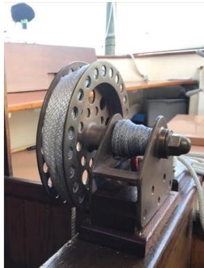
**Figure 10:** Racing style, antique centerboard winch aboard the catboat FAIRWEATHER
