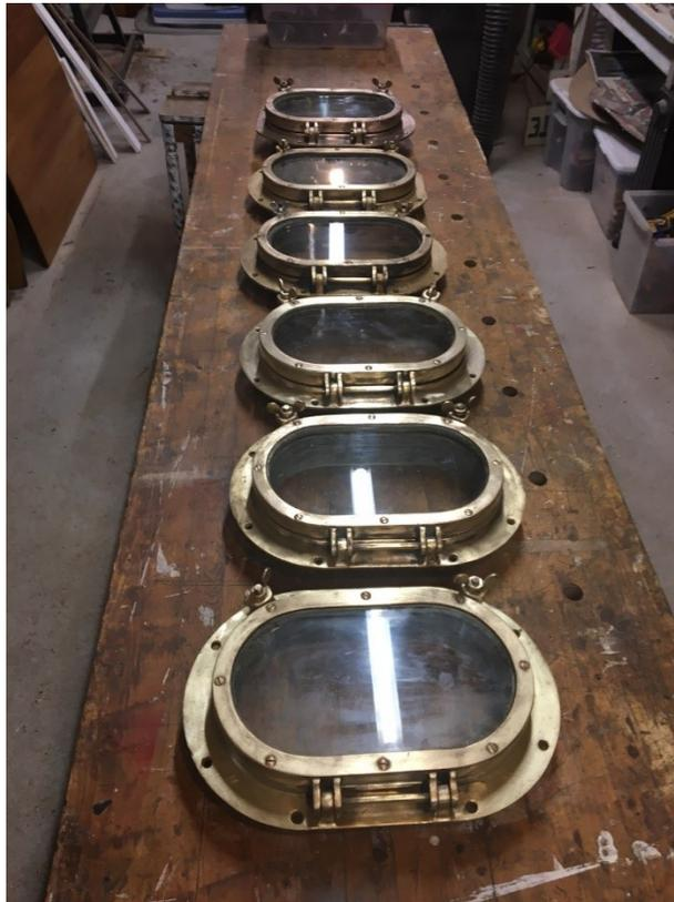
**Figure 19:** The refurbished and restored large portholes are ready to return to service.
