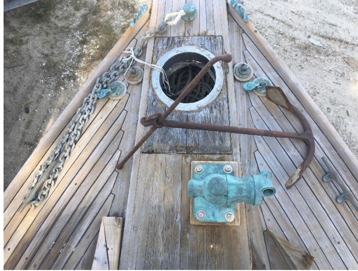
Figure 18: The new hawser pipe, line and chain should work well with the antique anchor.
