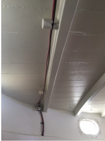
Figure 12: For historical reasons we rewired the running lights using the existing knobs.
