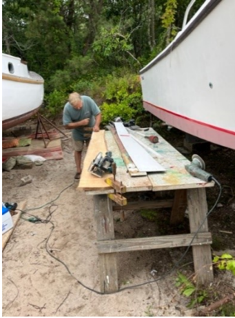
Photo 5: Bob used a template of the old garboard plank to fashion a new one
