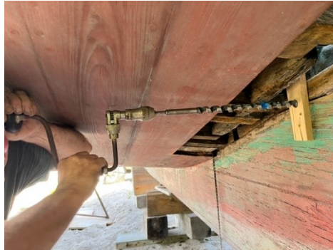
Photo 3: Bob drilling new stopwater holes with a bit brace and auger
