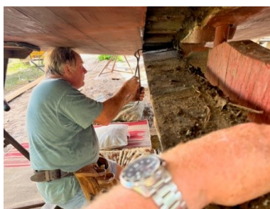
Photo 1: Bob Luckraft removing the port garboard plank
