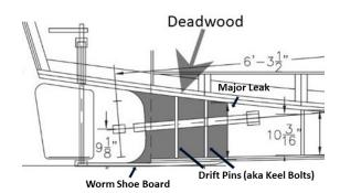
Repair will unfortunately require us to once again haul SUSPECT out of the water. It will involve removal of a portion of her worm shoe to expose the ends of the drifts. Once the drifts are visible we will be able to (hopefully) caulk and seal both them and the shoe. We can then arrange for a "third time's the charm" relaunch.
