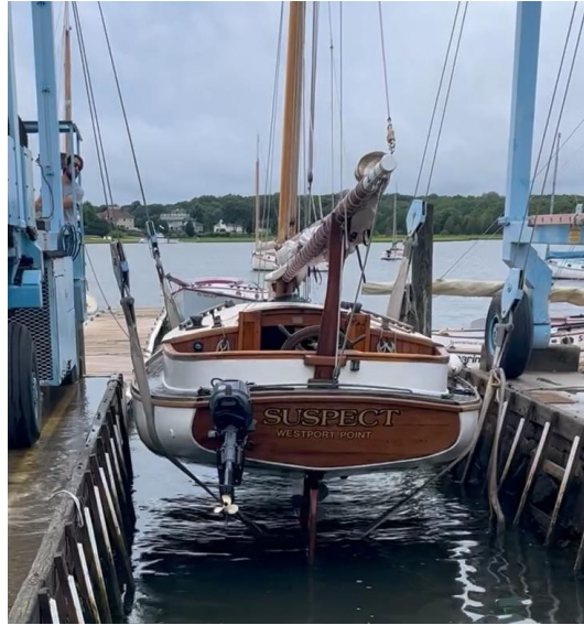
Figure 4: SUSPECT's open seams recaulking required a haul-out at the Marshall Marine yard.
