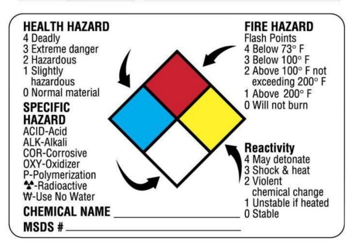
"The National Fire Protection Association (NFPA) uses a color-coded diamond to identify the hazards of a material.
