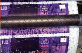
The cornerstone of SpeedFlex<sup>™</sup> end seals is a proprietary base material combined with an anti-friction insert, better known as a "rotary doctor blade". The primary structure of SpeedFlex<sup>™</sup> has superior compression/recovery properties that ensure intimate contact is maintained between the radius of the seal and the anilox roll circumference. The result is outstanding resistance to abrasive wear and hydraulic pressure applied by ink and cleaning solvents.
