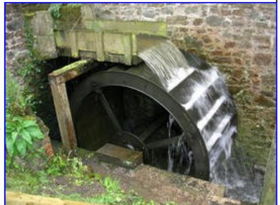
Overshot Wheel. This kind of mill requires a significant amount of fall to be practical, as the water must enter the wheel at the top. The Butler Mill was most likely not this classic design, as there is not enough fall between the mill pond site and the wheel.
