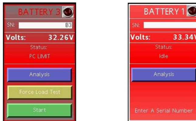
**Red gradient showing PC LIMIT (Left) and Solid red showing the estop was pressed (Right)**
