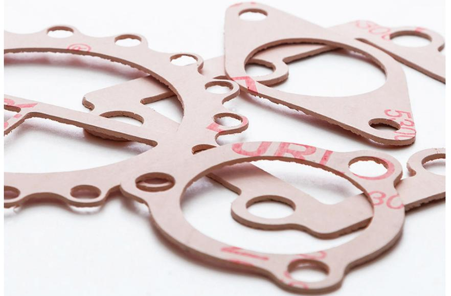
A good quality commercial grade compressed non-asbestos sheet for moderate service conditions suitable for steam, oil, water, mild alkalis, mild acids, hydrocarbons and solvents. Durlon® 5300 has the ABS Product Design Assessment Certificate (14-HS1146798-PDA) for intended service in marine and offshore applications.
