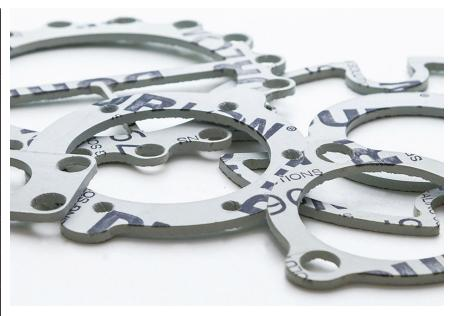
Durlon® 7900 is an economy grade general service gasket sheet material made with NBR (Nitrile Bonded Rubber) binder for mild service in piping and equipment with applications in steam, hydrocarbons and refrigerants and an alternative when temperature and pressure conditions are below 500°F (260°C) and 1200 psig (See PxT chart below for validation).
