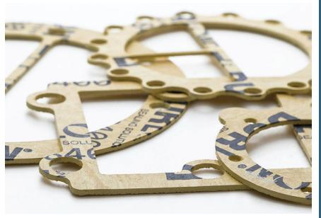
With an extremely wide pH application range (2-13 at room temp.) Durlon<sup>®</sup> 8400 can be used in process piping and equipment in chemical, pulp & paper and other general industrial applications. A unique high-performance compressed sheet, Durlon<sup>®</sup> 8400 is an excellent gasket material for use in steam, mild caustics and acids.
