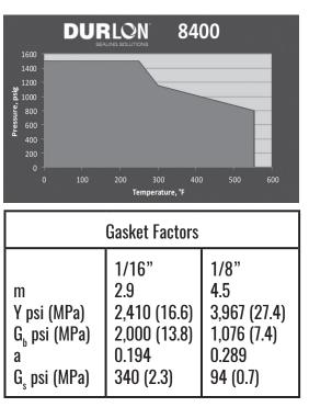
Anti-Stick Properties: Much effort has gone into improving the anti-stick release agents of all compressed Durlon<sup>®</sup> products. All Durlon<sup>®</sup> compressed gasket materials have passed the MIL-G-24696B Navy Adhesion Test (366°F/48hrs).
